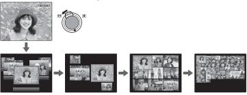
When two or more images are displayed, use the selector to highlight images and press **MENU/OK** to view the highlighted image full frame. In the nine- and hundred-frame displays, use the selector to view more pictures.
